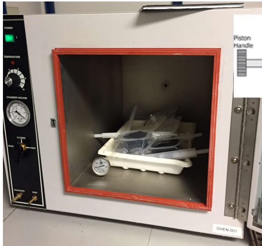
Incubation at elevated temperature – product in Tedlar bag
